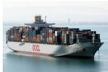
Example of container. 200,000DWT 400m X 59m X 33m, Draft 16m
