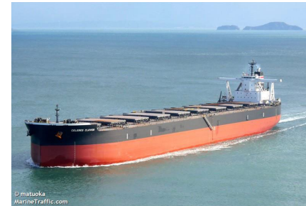
Example of bulk carrier. 210,000DWT 300m X 50m X 25m, Draft 18m
