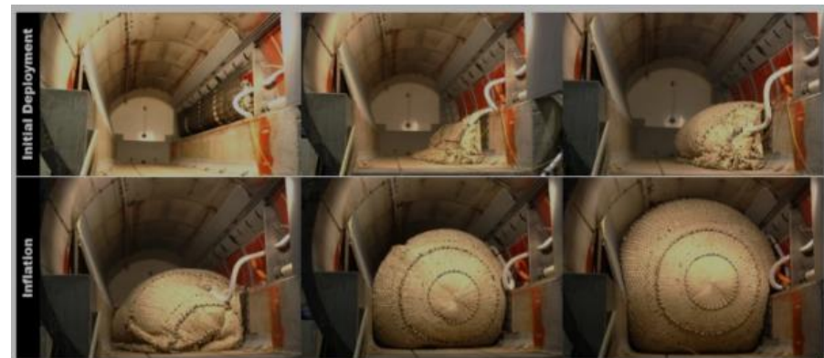
Phase 2b, full-scale testing, and three-layer Vectran plug. Deployment and low-pressure air inflation for the initial positioning of the plug before flooding simulation
