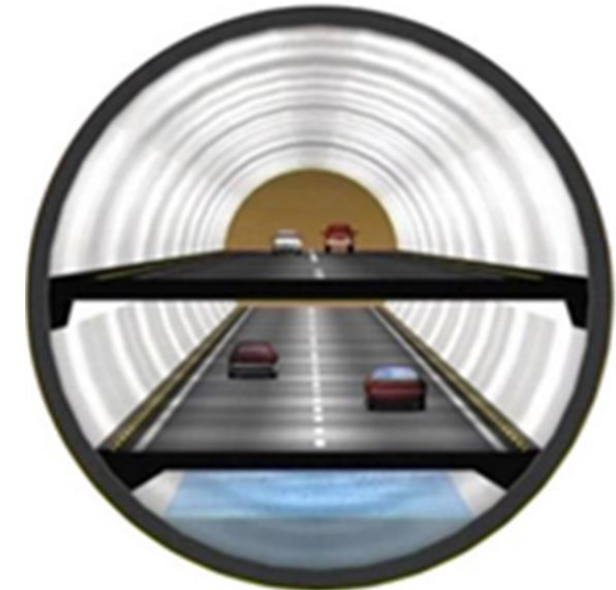
(Double deck, Slurry TBM)
