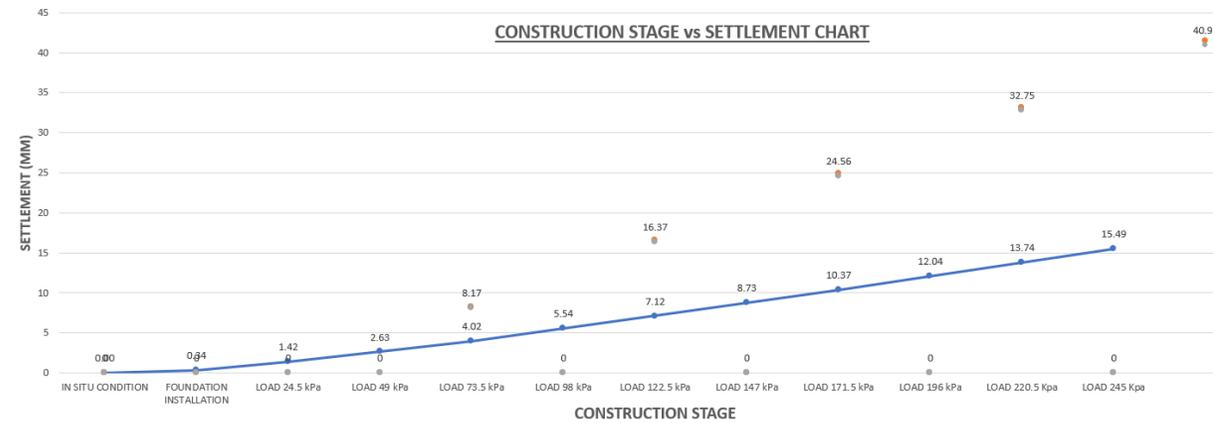
Hydrocarbon Tank Loading Stage Settlements
